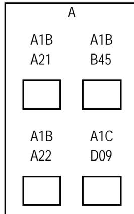
The above faceplate indicates that there are 3 cables coming from the A1B location, and 1 cable coming from A1C. The colour of the jack will indicate whether it is a data or voice connection. All of the faceplates must also be labelled with their position in the room to match the label on the cable, be that A, B, C, D etc. The locations start from the primary entry, then clockwise around the room. Refer to the table in **Section 4.7.3** for jack colour coding requirements.
