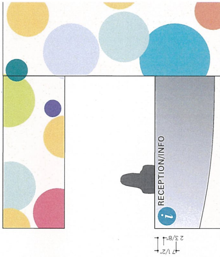
3A Area Identification - Reception Single sided, non-illuminated aluminum alupanel with vinyl text and graphics applied to face mounted to surface of reception desk. An optional thematic graphic application may accompany this identification sign to compliment the facility. Size: Dependant on reception desk design
